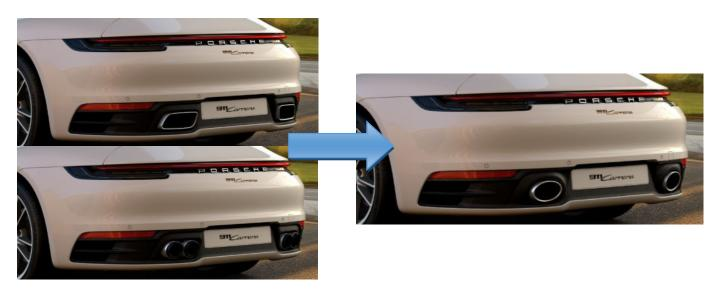
Following Porsche part numbers have to be ordered according to the region where the car is located as different regions use different license plate dimensions and as a consequence different diffuser part numbers.
