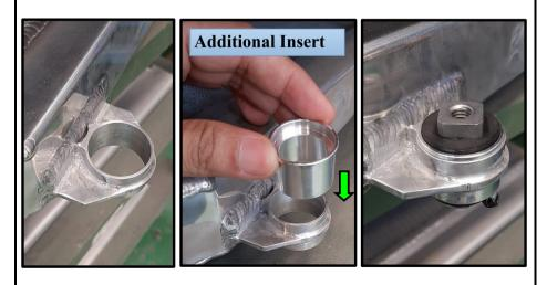
For 3rd Gen Tacomas (2016 +) use additional insert w/ smaller 22mm rubber mounts
